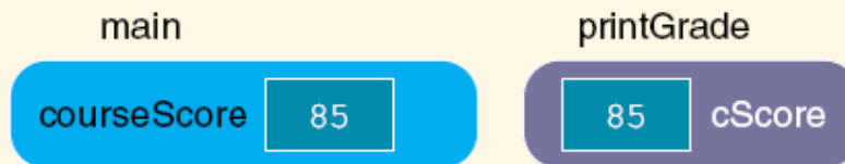
FIGURE 7-3 Variable courseScore after the statement in Line 6 is executed and control goes back to main
